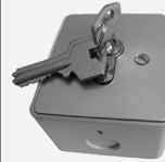
Art. nr. 504903 Standard control element for secure use of one to two drives. Die-cast metal housing with aluminium front plate, IP 54, design 2-sided pressing incl. Standard cylinder lock with 3 keys. double-keyed (NC contacts 300V, 5A), W70xH80xD47mm
