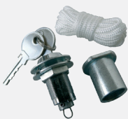
Art. nr. 504901 Plug-in lock for installation of all included emergency releases on doors without an interior turn handle. Maximum door panel thickness 48mm; a hole of 20 mm or 23 mm becomes necessary in the door panel.
